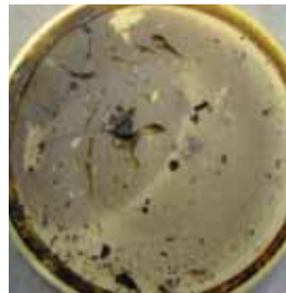
3" diameter Indium tin oxide target sputtered at 1000W (roughly 7x the maximum recommended power)
