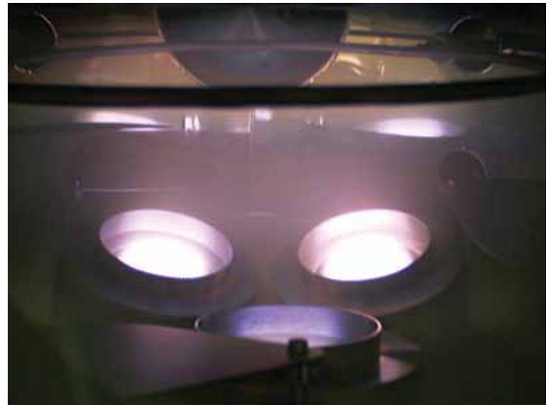
Sputter sources in co-deposition 'action'
