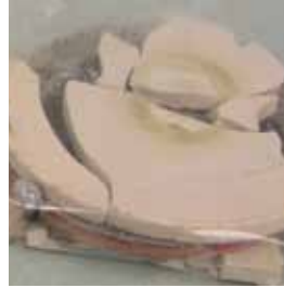
3" diameter Indium tin oxide target sputtered at 1000W (roughly 7x the maximum recommended power)
