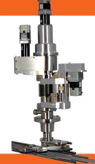
The 3-axis RTTA provides 360° rotation, 760mm linear extension and Z shift to provide arm lift/ lower to aid in sample transfer. Less than 1mm deflection at full arm extension with 10N load, linear reproducibility of <0.1mm and rotational reproducibility of <0.2mRad. Motorization options available.
